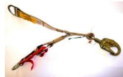
2. Check that stainless slide pin or cable is engaged through the nylon loop and into the aluminum tube retainer (slide pin) or fabric sleeve (cable) (see Fig."1" & "1A").
